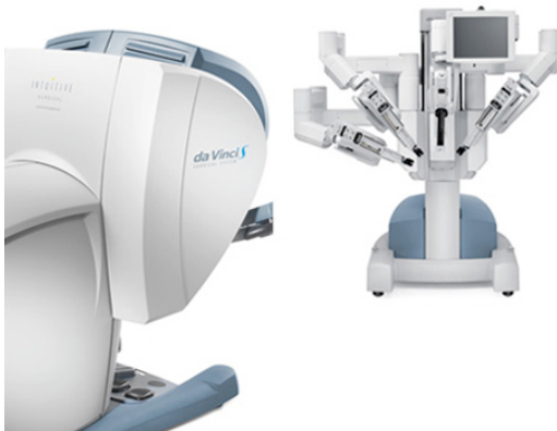
da Vinci Surgical System control console on left, robotic arms on right
