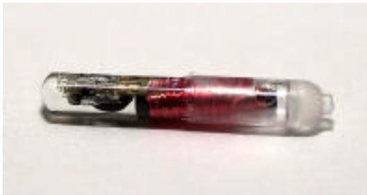
VeriChip: 12mm by 2.1mm or about the size of a dime
