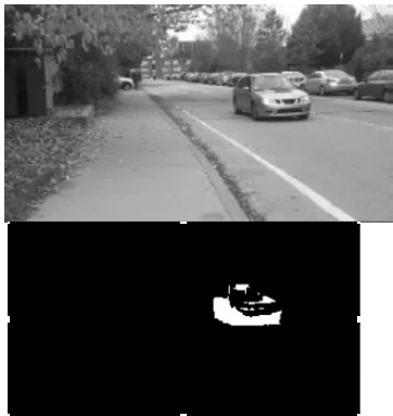
Figure: Top image shows original video, bottom image shows image after frame subtraction and filtering
