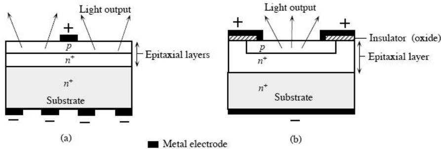
A schematic illustration of typical planar surface emitting LED devices. (a) p-layer grown epitaxially on an n<sup>+</sup> substrate. (b) First n<sup>+</sup> is epitaxially grown and then p region is formed by dopant diffusion into the epitaxial layer.
