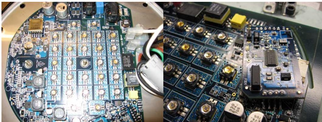
Following is a new version of the board. This board uses even smaller, but brighter LEDs. Heat dissipation is even more crucial. It can be seen that there is even more amount of copper and the LEDs are separated a little bit.
