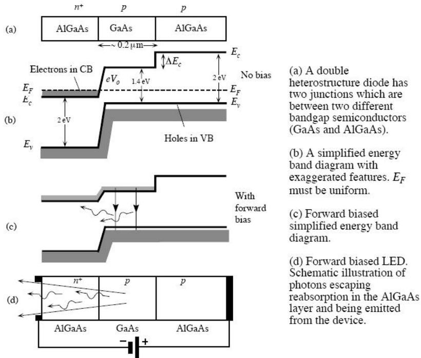
(a) A double heterostructure diode has two junctions which are between two different bandgap semiconductors (GaAs and AlGaAs).
