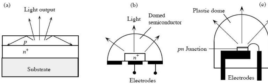
(a) Some light suffers total internal reflection and cannot escape. (b) Internal reflections can be reduced and hence more light can be collected by shaping the semiconductor into a dome so that the angles of incidence at the semiconductor-air surface are smaller than the critical angle. (c) An economic method of allowing more light to escape from the LED is to encapsulate it in a transparent plastic dome.
