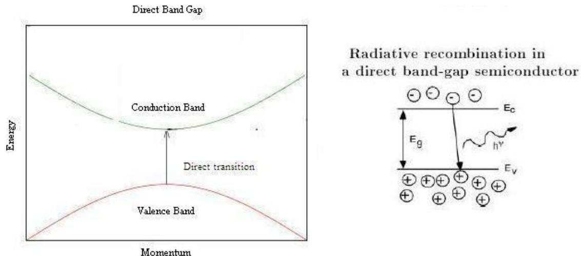
**Figure 2: Direct Bandgap and Direct Recombination**
