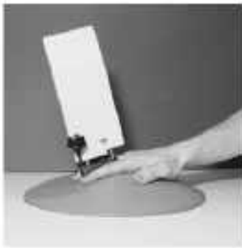
Figure 1 Prototype laser imaging system (without cover)
