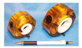
The robot is also nonmagnetic and dielectric, making it MRI safe as well. It is powered by the step motor. The robot is remote controlled using a computer. It is guided by an MRI, which is the preferred method of soft tissue imaging. The robot moves slowly but very precisely. It increases accuracy in collecting tissue samples for biopsy.
