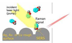
The difference in energy between the incident photon and the Raman scattered photon is equal to the energy of a vibration of the scattering molecule. A plot of intensity of scattered light versus energy difference is a Raman spectrum. The Raman spectrum provides a unique signature of the molecule acting like a fingerprint in identifying it. This is how it can be used to detect glucose however that is not the only use to come of this technology.
