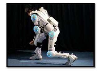
complications in the nervous system or in the muscles, the HAL robotic suit has the ability to utilize other signals, such as the FRF (floor reaction force), joint angles, and shifts in the patient's center of gravity to determine the desired motion.
