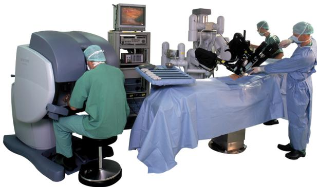
The patient side cart provides either three or four robotic arms—two or three instrument arms and one endoscope arm, that execute the surgeon's commands. The laparoscopic arms pivot at the 1-2 cm operating ports, eliminating the use of patient's body wall for leverage and minimizing tissue damage. Supporting surgical team members assist in installing the proper instruments, prepare the 1-2 cm port in the patient and supervise the laparoscopic arms and tools being utilized.
