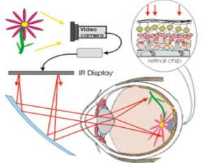
The Future goals in this field are to make the entire device fully implantable. Currently the camera, image-processing hardware, power amplifier, and data modulator are external hardware. The first and most difficult part of this is making a miniaturized camera that can fit on the lens of the eye. Hopefully all of this hardware will become small enough to fit onto the lens of the eye and hopefully be invisible.
