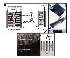
A specific super capacitor has been designed and tested with very good success at MIT. This design features cellulose as the insulator for the capacitor. Multiwalled nanotubules that act as electrodes are combined with the cellulose. The final component is the electrolyte. This can be an ionic aqueous solution such as blood or a non aqueous ionic electrode. The end result is an extremely flexible energy source that can withstand a wide range
