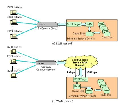
Figure 1. Experimental settings for performance measurements of iSCSI remote mirroring.
