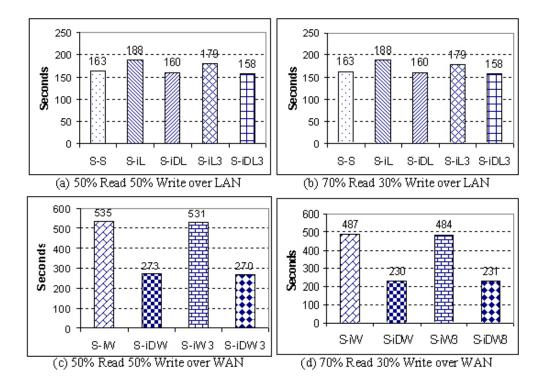
Figure 2. PostMark results: total time to finish 100,000 transactions on 10,000 files
