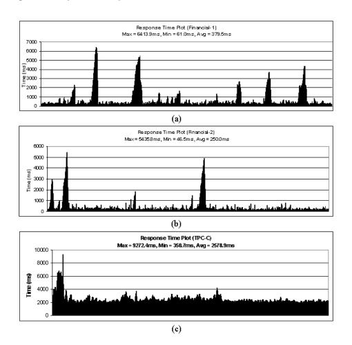
Figure 6. Response time with write coalescing (batch size=8 consecutive writes) over WAN.
