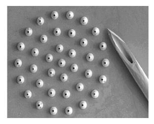
An array of hollow microneedles compared to a traditional hypodermic needle.
