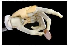
The ability of the i-LIMB to articulate each finger individually literally and figuratively opens doors for amputees. Patients using other prosthetic hands would never be able to maneuver a key into a key hole to unlock a door. This is only one of the many fine motor skills that this device allows patients to complete.
