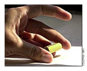
The company's system incorporates several technological breakthroughs that have only recently appeared on the market. The tiny imaging system can only have been made possible with the improvement of the signal to noise ratio in CMOS detectors, development of white LEDs, and development of application-specific integrated circuits (ASICs).
