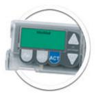
The pump is intended to be used continuously and delivers insulin 24 hours a day according to a programmed plan unique to each pump wearer. The pump mimics the pancreas by giving a small amount of insulin continually (the "basal rate"). This insulin keeps blood glucose in the desired range between meals and over night. When food is eaten, the user programs the pump to deliver a "bolus dose" of insulin matched to the amount of food that will be consumed.
