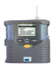
The electronic nose consists of two components an array of chemical sensors (usually gas sensors) and a patternrecognition algorithm. The sensor array "sniffs" the vapors from a sample by taking samples of the chemical composition and provides a set of measurements and the pattern-recognizer compares the pattern of the measurements to stored patterns for known materials. The E-Nose is useful for numerous tasks concerning sensing the presence of chemicals.
