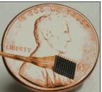
The silicon electrodes can read the electrical signal (impulses) of when and how neurons are fired.
