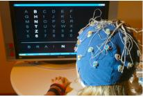
Results showed that of all test subjects, an average of 65% of all letters were transferred correctly through EEG signals to the output device.
