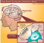
This device is connected to a person's head, whether invasively or un-invasively, and works to relay a signal to a computer. The P300 BCI monitors conscious brain activity through EEG signals, and then uses digital signal processing algorithms to turn these signals into commands. Simply put; there is an input, a pattern recognition algorithm, and an output.
