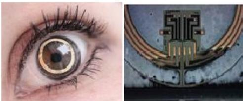
When the eye fills with fluid the diameter of the cornea changes and this information is collected by the strain gauge. This data is then processed and sent to the antenna which then sends radiofrequency waves back powering the lens. Once the data is collected it can then be transmitted to a doctor's computer via Bluetooth for a full analysis.
