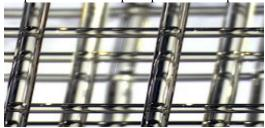
network. Once the template was created by the 3-D printer, living cells were inserted and grown into the desired network shaped. After the network had finished developing, the sugar template was dissolved. The template created by the researchers can be seen in the figure above.
