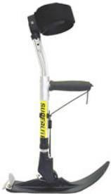
The monoski contains 4 main parts, a molded seat, a footrest, a frame, and a ski. The frame is made of aluminum and steel. It contains a boot that attaches to the ski and a suspension unit that absorbs shock, keeps the ski edges on the ground for better control, and connects to the seat and footrest. The seat is the equivalent of the ski boot to stand up skiers. It attaches your body to the ski and requires a good fit. The seat is made of composite materials and foam and has
