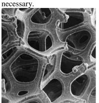
Here is a picture of the metal foam as you can see it has many interconnecting pores that make it easy for the blood vessels and bone cells to grow into. When comparing the design of the metal foam to that of a normal bone the structures are nearly identical.
