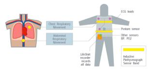
Above: VivoMetric's *LifeVest*'s sensor placement in their smart textile. Most other smart textiles use this same placement in order to obtain the best results. Sensatex's *Smart Shirt* also uses the same set-up of sensors, except this piece of biomedical technology is mainly used for obtaining vitals for military use.
