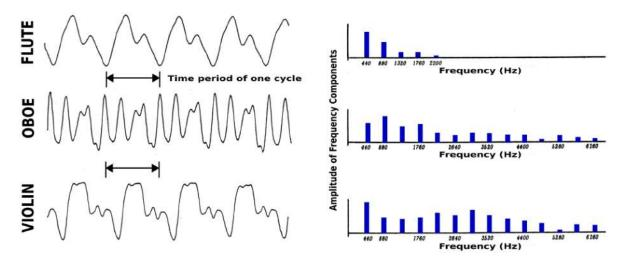
The time period of one cycle shown in the figure is the reciprocal of the fundamental frequency:
