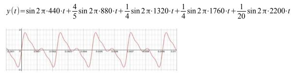
While the simulated waveform bears the general shape of the actual waveform, there is some degree of discrepancy. This may be due to unrepresented *phase* components, which are time delays among the different harmonics. The effect of the phase will be further discussed later.
