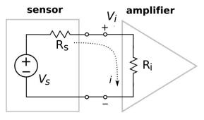
For maximum power transfer,  $R_i$  should match  $R_s$ .:
