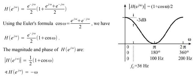
The system has a linear phase response, which represents a group phase delay. The linear phase is desirable because it does not introduce any *phase distortion*.
