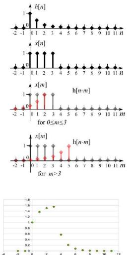
This is a low-pass filter. For the square pulse input, the output is a charge-discharge curve that shows reduction of the high-frequency contents. Example 2. We implement a 3-point FIR low-pass filter to smooth the data according to:
