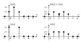
Because convolution in the time domain is equivalent to multiplication in the frequency domain, the overall transfer function is the product of the individual transfer functions.
