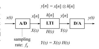
The sampling rate  $f_s$  set forth by the A/D is arguably the most crucial parameter in this digital system. Sampling is almost always done periodically with a sampling period of T.
