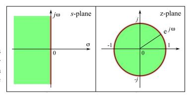
The Fourier transform is the ZT evaluated on the unit circle. The Fourier transform (FT) and the inverse Fourier transform (IFT) are defined as follows:
