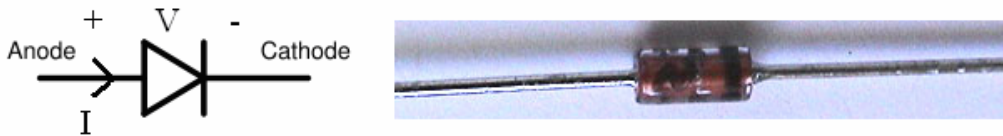
Figure 5. Diode schematic symbol and actual picture of a common 1N914 diode (the black stripe in the picture is the cathode). Conventional current can flow from the anode to the cathode, but not the other way around. Notice that in EE, the Anode is the positive terminal and the cathode is the negative terminal.
