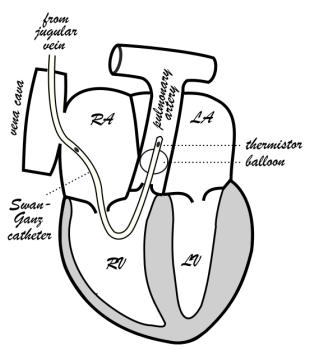
Consider the following example: The cardiac output is determined by use of the thermodilution method. A bolus of 24 ml iced saline (0 °C) was rapidly injected into the right atrium. The temperature is measured in the pulmonary artery as shown on the right. Assume a heat loss factor of 0.85. Determine the cardiac output in terms of liters per minute.
