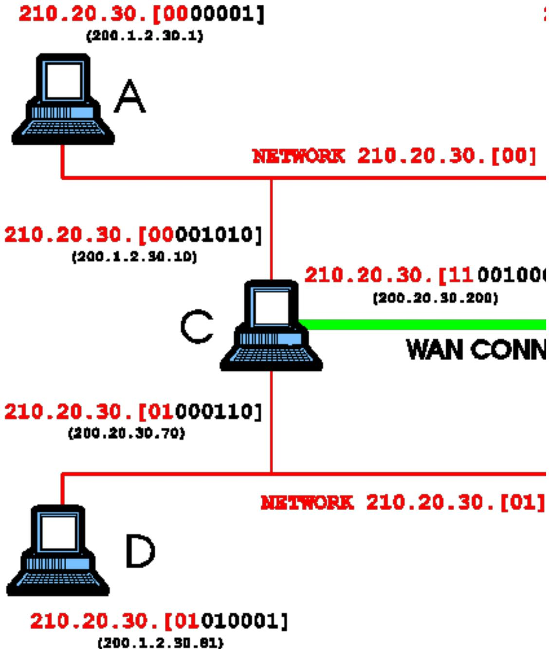
We have expanded the last byte of the IP address so that we can show the network subaddressing. The standard IP address nomenclature is shown below this expanded version.
