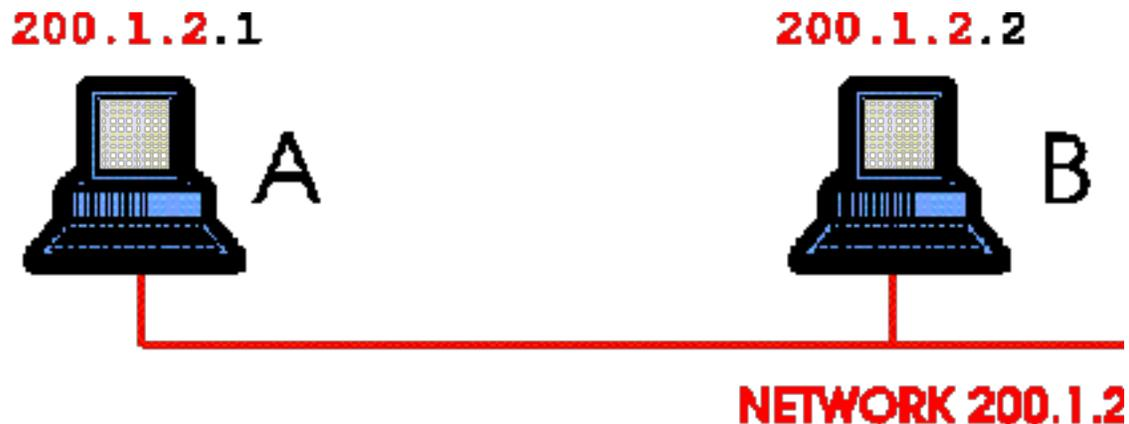
In the diagram above and subsequent diagrams, we have emphasized the network number portion of the IP address.
