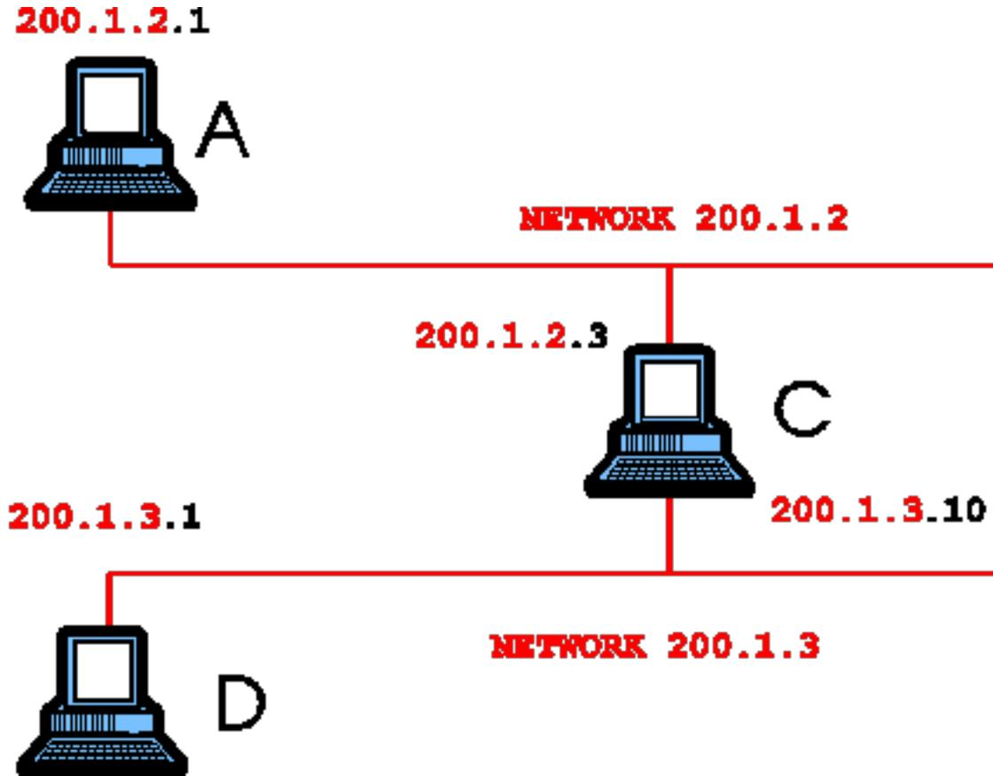
Device C is acting as a **router** between these two networks. A router is a device that chooses different paths for the network packets, based on the addressing of the IP frame it is handling. Different routes connect to different networks. The router will have more than one address as each route is part of a different network.
