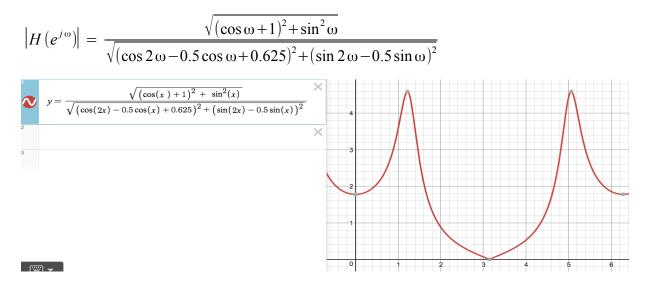
The system is substantially underdamped as indicated by the prominent peak, which is related to the two poles close to the unit circle.
