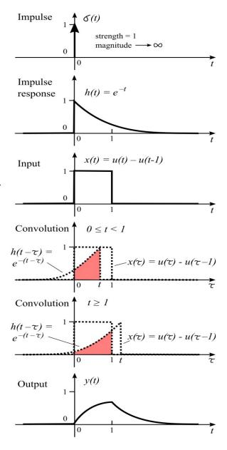
Convolution in the time domain is equivalent to multiplication in the frequency domain. The figure shows the LTI system in the frequency domain. H(s) is the transfer function, which is the Laplace transform of the impulse response h(t). H(s) is the ratio of the LT of the output over the LT of the input:
