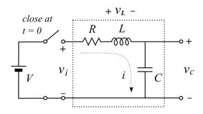
be completely characterized by its impulse response h(t). The step response is the convolution between the input step function and the impulse response:  $s(t) = u(t) \otimes h(t)$ .
