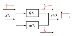
Example 3: Using the same F(s) and G(s), what is the overall transfer function H(s) if the two are connected in series?
