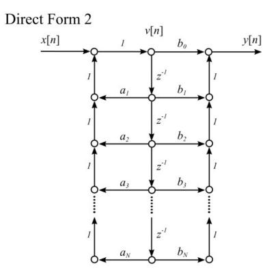
The validity of Direct Form 2 is not immediately obvious. Thus, we will prove that the Direct Form 2 does result in the same transfer function. Let v[n] be the intermediate signal as shown above.
