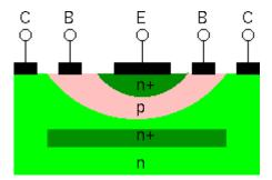
Figure 1: Cross section of an NPN Transistor
