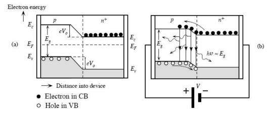
(a) The energy band diagram of a  $pn^+$  (heavily n-type doped) junction without any bias. Built-in potential  $V_o$  prevents electrons from diffusing from  $n^+$  to p side. (b) The applied bias reduces  $V_o$  and thereby allows electrons to diffuse or be injected into the p-side. Recombination around the junction and within the diffusion length of the electrons in the p-side leads to photon emission.
