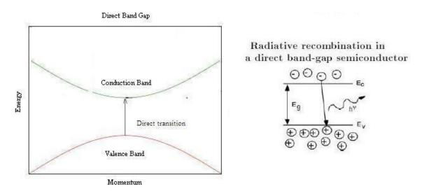
Figure 2: Direct Bandgap and Direct Recombination
