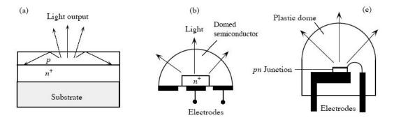
(a) Some light suffers total internal reflection and cannot escape. (b) Internal reflections can be reduced and hence more light can be collected by shaping the semiconductor into a dome so that the angles of incidence at the semiconductor-air surface are smaller than the critical angle. (b) An economic method of allowing more light to escape from the LED is to encapsulate it in a transparent plastic dome.
