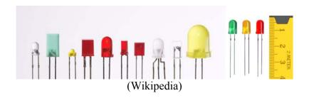
Most LEDs were made in the very common 5 mm T1-3/4 and 3 mm T1 packages, but with higher power, it has become increasingly necessary to eliminate the heat, therefore the packages have become more complex and adapted for heat dissipation. Packages for state-of-the-art high power LEDs bear little resemblance to early LEDs. For example, the following picture shows a Philips Lumiled LUXEON K2.
