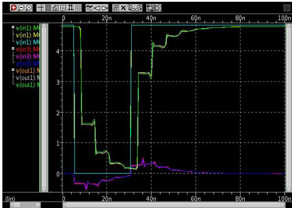
Figure 45 Monte Carlo Analysis with Field Solver and W-element
