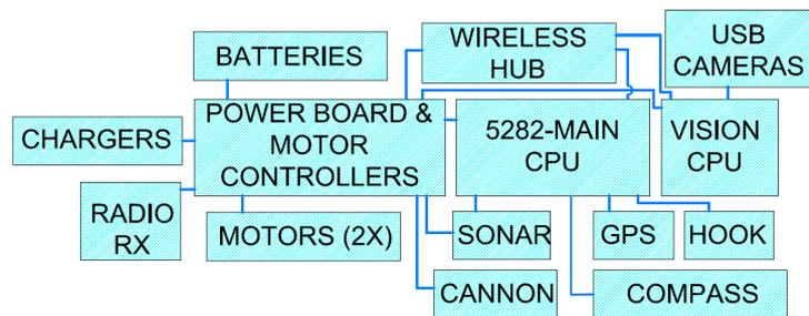
Figure 3: ASV subsystems block diagram
