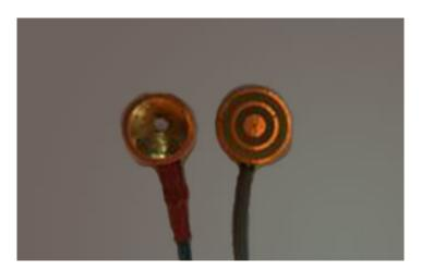
Walt Besio developed a tripolar ring electrode, which is compared to a conventional electrode. Credit and Larger Version
