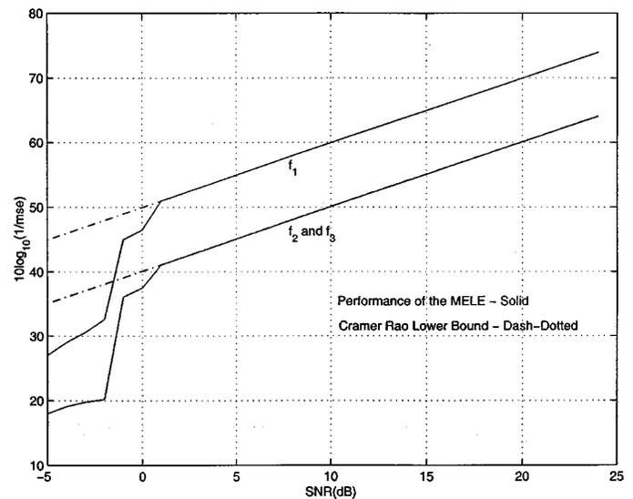
Fig. 8. Performance of the mean likelihood estimator for three sinusoids in additive white Gaussian noise.
