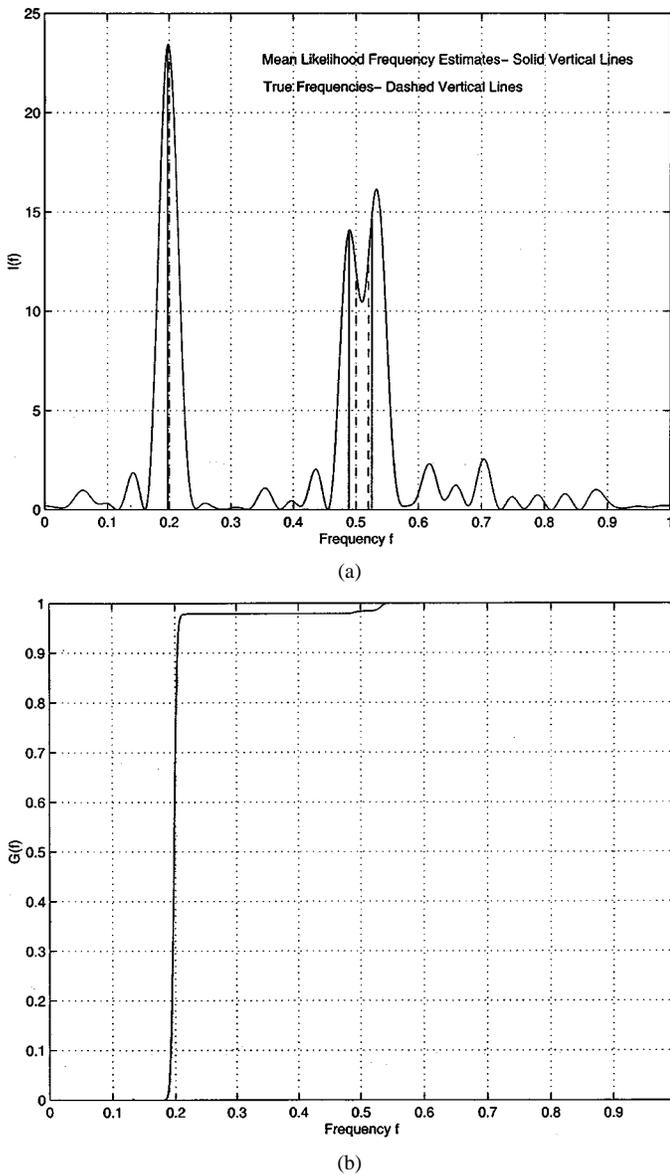
Fig. 7. (a) Periodogram of the data for three sinusoids in additive white Gaussian noise, SNR = 5 dB. (b) Plot of cumulative distribution function  $G(f)$  for the three-sinusoid case, SNR = 5 dB.
