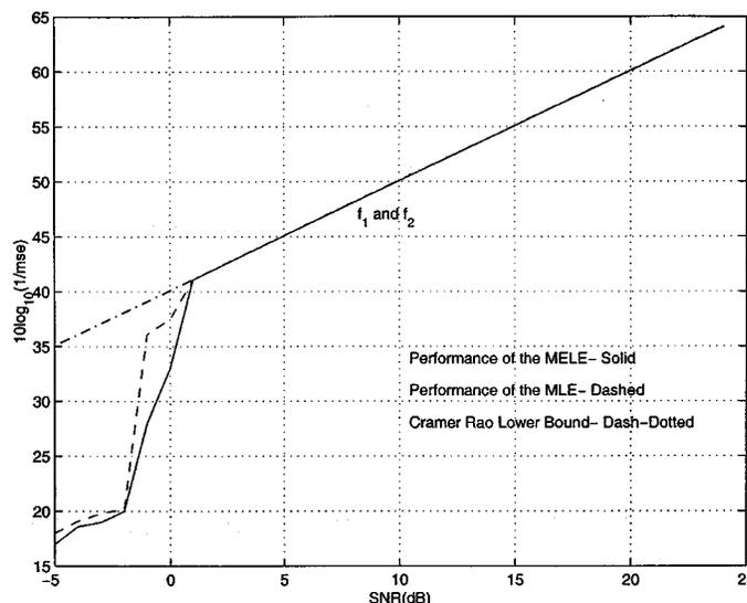
Fig. 5. Performance of the mean likelihood estimator for two sinusoids in additive white Gaussian noise.
