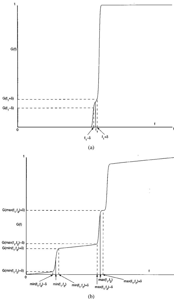
Fig. 3. (a) Generation of frequency  $f_2$  for two sinusoids. (Generate  $u_2 \sim U[(0, G(f_1 - \delta)) \cup (G(f_1 + \delta), 1)]$ , where  $f_1 = G^{-1}(u_1)$ ). (b) Generation of frequency  $f_3$  for three sinusoids. (Generate  $u_3 \sim U[(0, G(\min(f_1, f_2) - \delta)) \cup (G(\min(f_1, f_2) + \delta), G(\max(f_1, f_2) - \delta)) \cup (G(\max(f_1, f_2) + \delta), 1)]$ , after  $f_1$  and  $f_2$  have been generated with the condition  $|f_1 - f_2| > \delta$ ).
