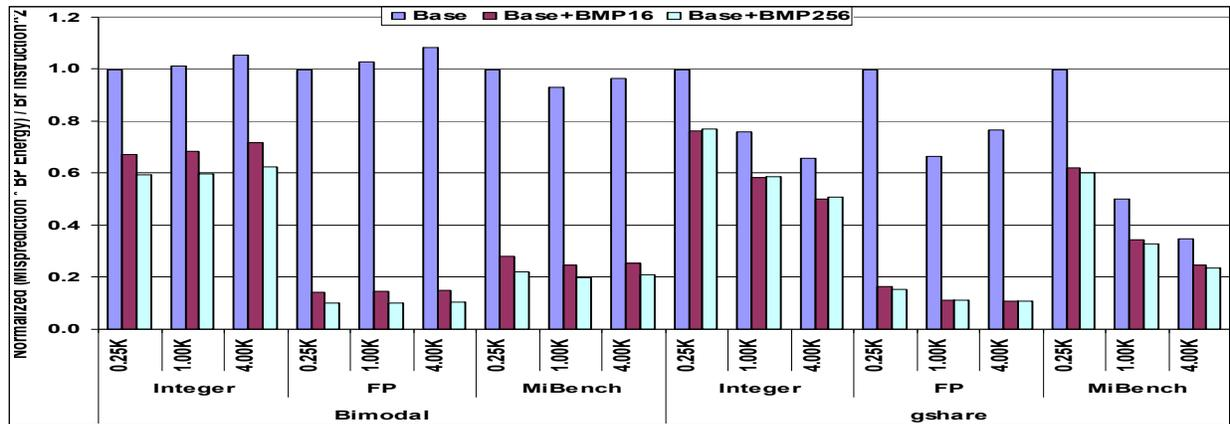
**Figure 12.** Improvement in branch predictor energy-efficiency due to adding a BMP. In the figure, lower is better.
