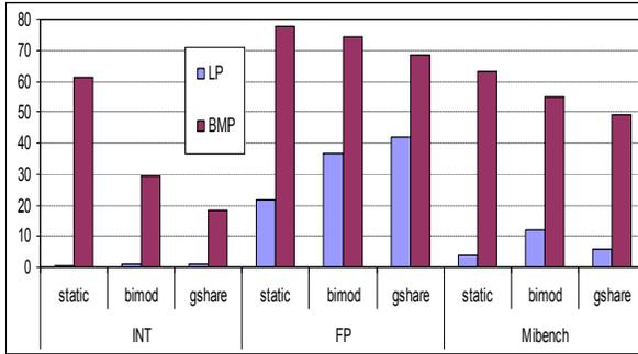
**Figure 10.** Percentage reduction in the branch misprediction rate with a 128 byte loop predictor (LP) or BMP. The sizes of the baseline dynamic branch predictors are 1KB.
