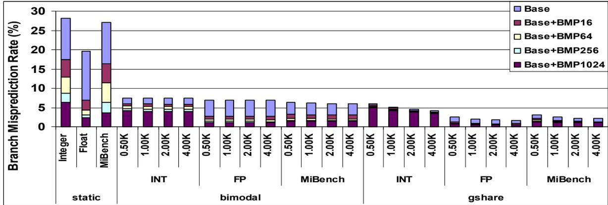
**Figure 6.** Reduction in the branch misprediction rate due to adding a BMP. The height of each bar represents the average branch misprediction rate without a BMP while the height of each segment shows the number of additional branch mispredictions that were removed by adding BMP entries. In this figure, smaller is better.
