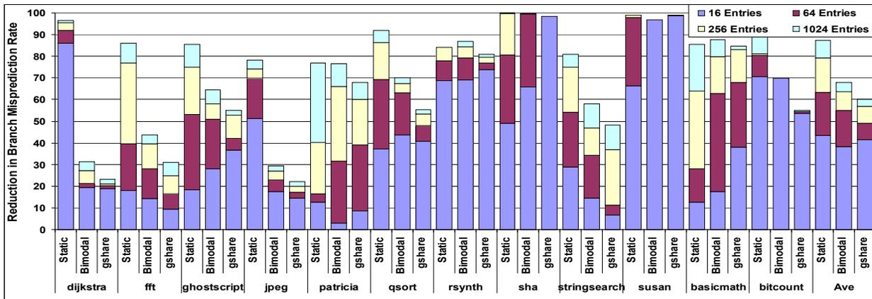
**Figure 9.** Percentage reduction in branch misprediction rate with BMP (baseline bimodal or gshare branch predictor is 1KB) for MiBench benchmarks.
