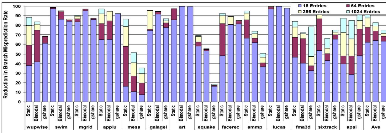
**Figure 8.** Percentage reduction in branch misprediction rate with BMP (baseline bimodal or gshare branch predictor is 1KB) for SPECfp 2000 benchmarks.
