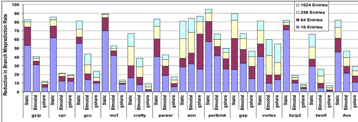
**Figure 7.** Percentage reduction in branch misprediction rate with BMP (baseline bimodal or gshare branch predictor is 1KB) for SPECint 2000 benchmarks.
