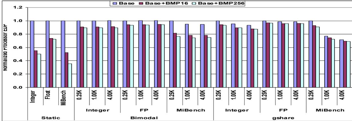
**Figure 13.** Improvement in processor energy-efficiency due to adding a BMP
