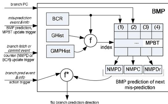
**Figure 1.** BMP components and operation. For simplicity, this figure only shows major components.  $f$  is logic that generates the MPBT index while  $f^*$  intervenes to correct potential mispredictions. Note that the MPBT is only accessed and updated after a mispredicted branch, and the BCR and the NMPD are updated on committed and fetched branches, respectively.
