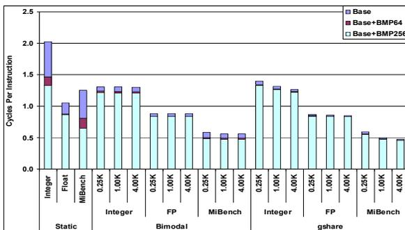
**Figure 11.** Reduction in CPI due to adding a BMP
