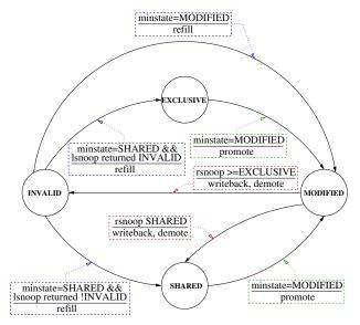
Fig. 2: Z4800 MESI state machine. 'Isnoop' refers to a locally-initiated snoop request; 'rsnoop' refers to a remotely-initiated snoop request. 'minstate' refers to the minimum state required to satisfy the outstanding local miss.
