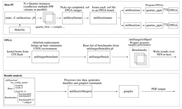
Fig. 4: Diagram of automated hardware synthesis/benchmarking system.
