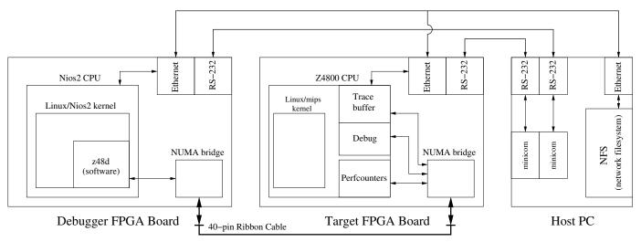
Fig. 3: Block diagram of debug setup using two Altera DE2-70 boards.
