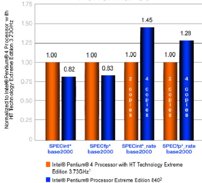
Figure 1. Intel single vs. multi-core performance.
