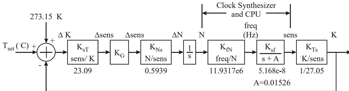
Figure 2. Single sensor, single feedback path control system.
