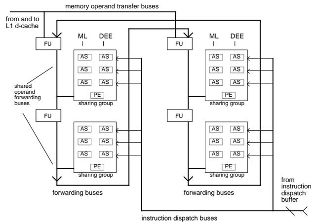
Figure 2: *The Execution Window.* Shown is a layout of the Active Stations (AS) and Processing Elements (PE) along with some bus interconnections to implement a large, distributed microarchitecture. Groups of ASes share a PE; a group is called a *sharing group*.
