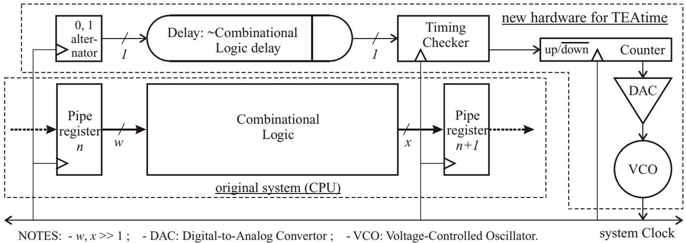
Fig. 1. Timing Error Avoidance (TEAtime) block diagram
