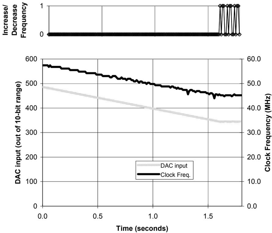
Fig. 8. Experiment 1, part B: Decreasing-frequency stabilization.
