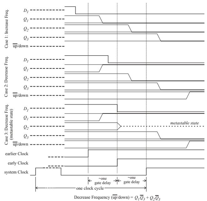
Fig. 4. Timing Checker / TEAtime detailed timing.
