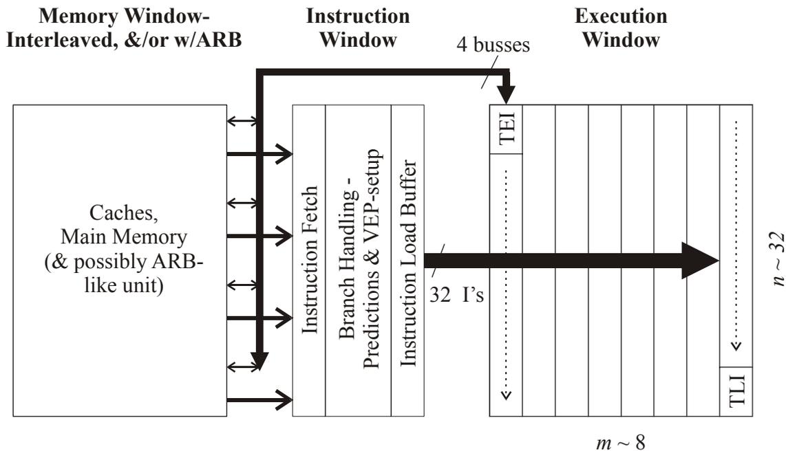
**Figure 2 Levo block diagram. In order to sustain a high IPC, many instructions must be fetched and loaded into the Execution Window simultaneously. (TEI – Temporally Earliest Instruction; TLI – Temporally Latest Instruction)**
