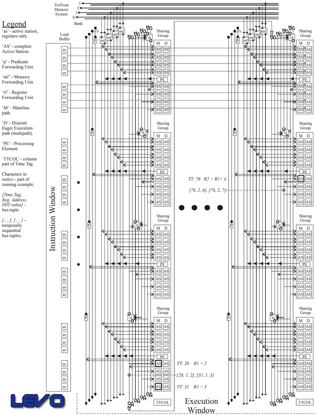
**Figure 3 Levo Execution Window details.** Two of possibly very many (*m*) columns shown. Number of rows (*n*) set to 32 and other dimensions set to specific values only for sake of illustration. A running example of operand broadcasting and snarfing is shown with *italics*: see the Legend. The example continues in Figure 4 and Section 3.1.6. The DEE AS's are not included in the simulation studies presented herein, but are left for future work. The point is, we know how to realize DEE in Levo.
