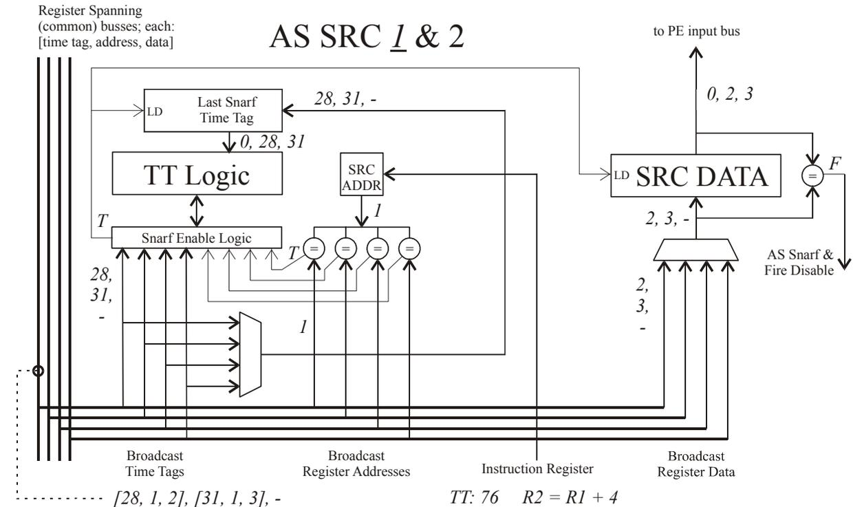
**Figure 5 AS Source Operand Logic.** Broadcast data is snarfed and the instruction is fired when its register address is the same as the SRC ADDR, and the broadcast time tag is less than this AS's time tag (implicit), and the broadcast time tag is greater than or equal to the time tag of the previously (Last) snarfed data, and the broadcast data differs from the current SRC DATA. Four spanning busses assumed (typical). Running example information in *italics* (see Figure 3 and Figure 4).
