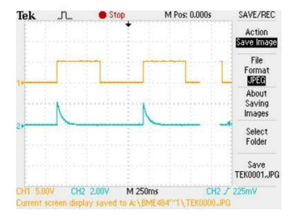
Figure 7: Channel 1 displays the square wave outputs from RC0. Channel 2 shows the output of the two stage gains which is fed to the input of the PIC (pin 2).
