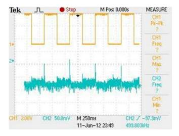
Figure 5: Channel 1 displays the square waves while Channel 2 displays the output of the voltage follower.
