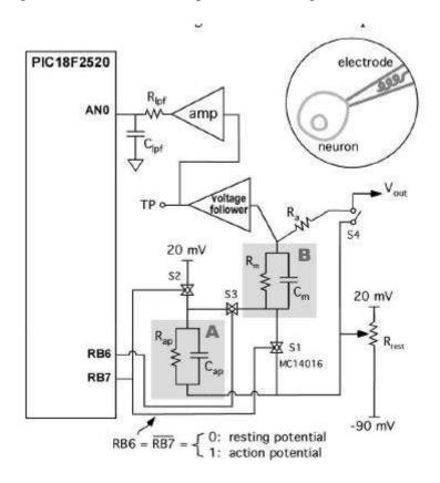
Figure 1: Schematic of the neuron emulator.
