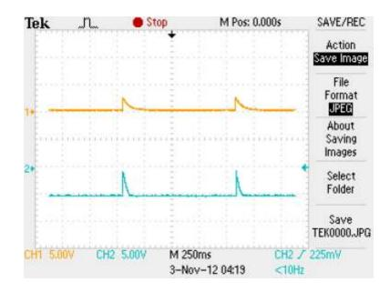
Figure 8: Channel 1 exhibits the input to the PIC while channel 2 is the output of the DAC.
