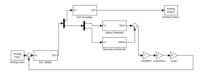
Figure 6: Block diagram of the current neuron emulator.
