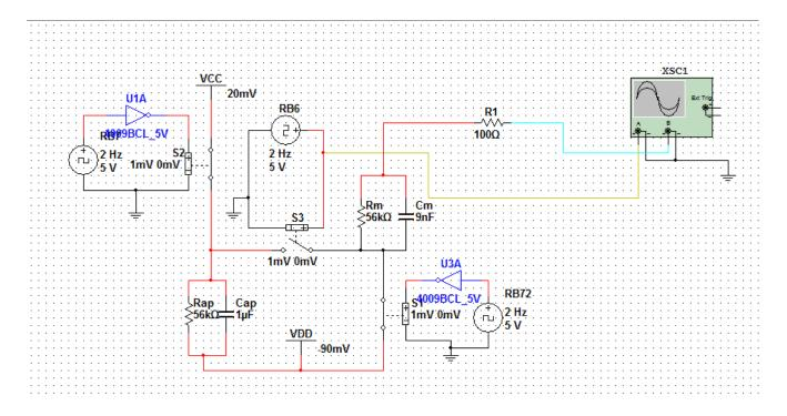
Figure 2: The neuron emulator simulated in MultiSim.
